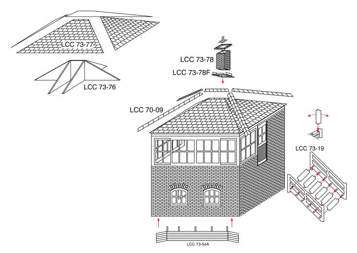
Remove roof support parts LCC 73-76 from their spruce and glue together by slotting together as shown on picture above. Leave them until glue dries prior making sure they are all at right angles to each other. Take out LCC 73-77 roof panels from their spruce and start gluing them to the supports. Assemble on a flat surface ensuring the roof is square on edges and flat on the bottom.
